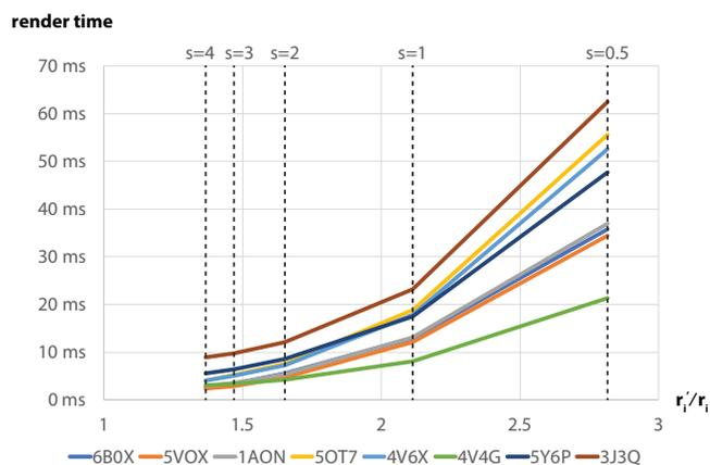
**Figure 10:** Scaling of the total render time with increasing sphere of influence radius according to Equation 8 for a viewport size of  $1280^2$ .
