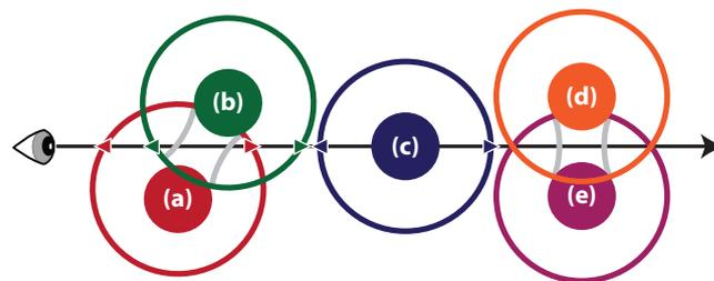
**Figure 2:** Illustration of our intersection list generation pass. The Gaussian surface can only occur where two or more spheres of influence (indicated by the outer circles) overlap, as is the case for the red (a) and green (b) spheres. Overlaps located behind a van der Waals sphere (indicated by the filled inner circles) do not need to be considered, so the orange (d) and purple (e) spheres are not stored in the list for the depicted ray, as they are occluded by the blue sphere (c).
