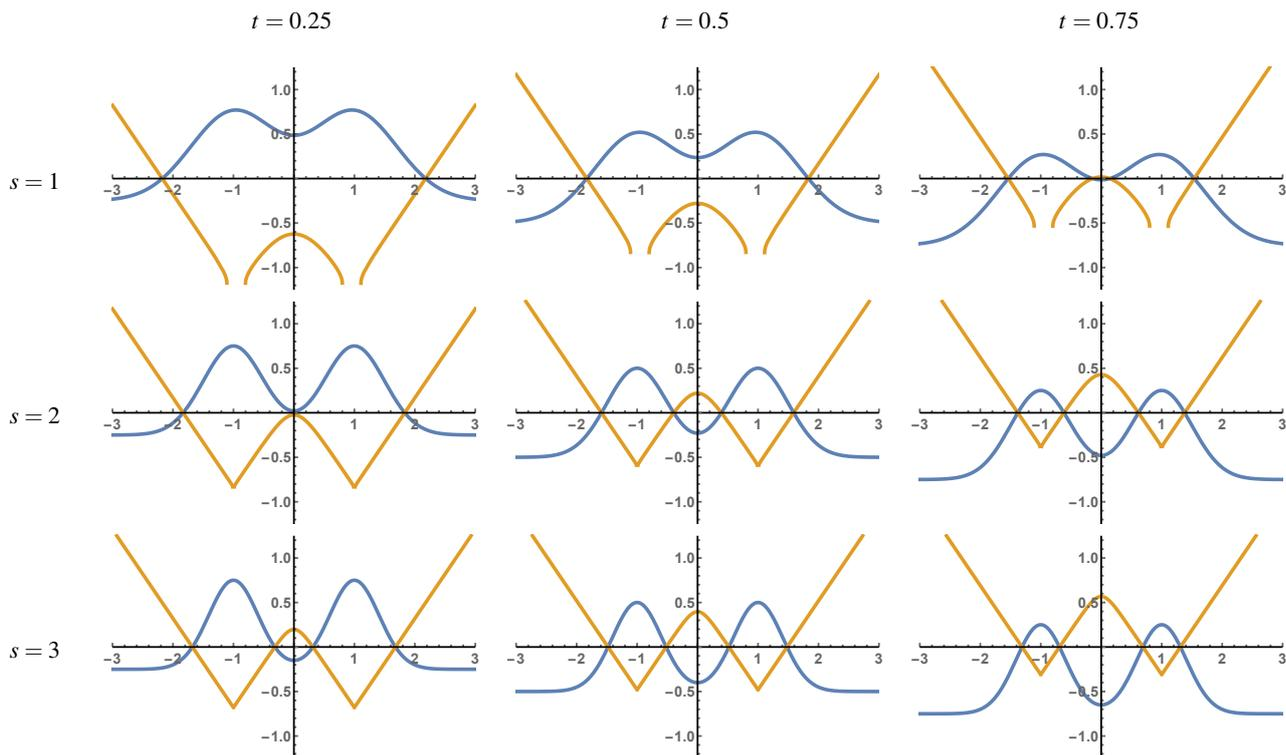
**Figure 3:** Plots of the Gaussian density function  $\rho(\mathbf{x}) - t$  (in blue) and the corresponding distance function  $\hat{\rho}(\mathbf{x}) - \hat{t}$  (in orange) for different values of  $s$  and  $t$  for two atoms positioned at  $-1$  and  $1$ . As can be seen, the behavior of the distance estimate is close to linear, and the roots of both functions are the same.
