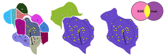
Figure 4. Clustering based on varying kernel sizes. Left: too small kernel, s(\phi) = 0.63 ; Middle: optimal size, s(\phi) = 0.72 ; Right: too big kernel, s(\phi) = 0.64 .
