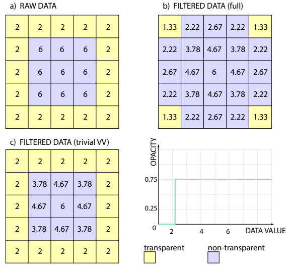
Figure 5: a) is a 2D projection of a noisy object. We use a simple averaging kernel 3 \times 3 . b) Full filtering that includes also transparent regions (background) and we consider it the ground truth. c) The result if we filter on non-transparent regions.
