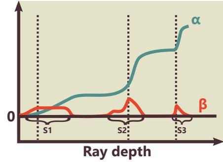
Figure 4: Borders of structures  $S_k$  are detected by local maxima of  $\beta$ . This defines a point cloud for the whole scene which is used for widget fitting.
