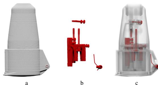
Figure 18: Using standard volume rendering methods the transfer function can be set to (a) show the outer geometry, to (b) show the inner structures, or to (c) show both using transparency.
