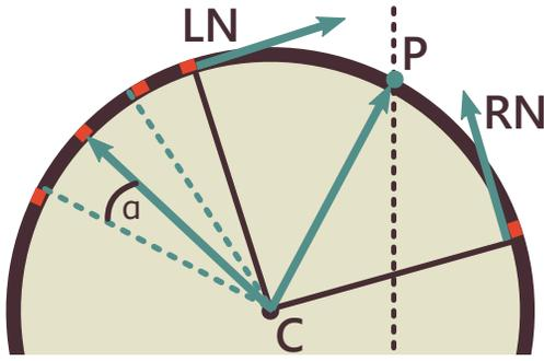
Figure 13: To compute the positions of the interaction tools on the sphere, we construct a vector  $CP$  and compute the dot product with normalized vectors  $LN$  and  $RN$  to estimate if the point  $P$  lies in the focus region defined by the user interface tool.
