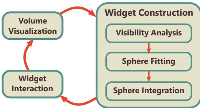
Figure 3: Overview of our approach for smart surrogate widgets and its integration into the volume visualization pipeline. To fit the surrogate widget into the rendered image, we analyze the visibility and compute a set of prominent points for the given visualization state. In the next step, we fit a sphere into the computed point set. The new sphere is combined with the existing widget. The updated widget can be used for further volume manipulation.
