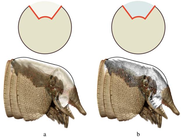
Figure 11: The upper row shows a simplified cross section of the widget. The upper part of the armadillo is covered with a smart surrogate widget consisting of two spheres. Through a combination of cones and wedges it is now possible to look into the body by reducing the opacity inside the widget using (a) the initial transfer function or (b) the alternate transfer function.
