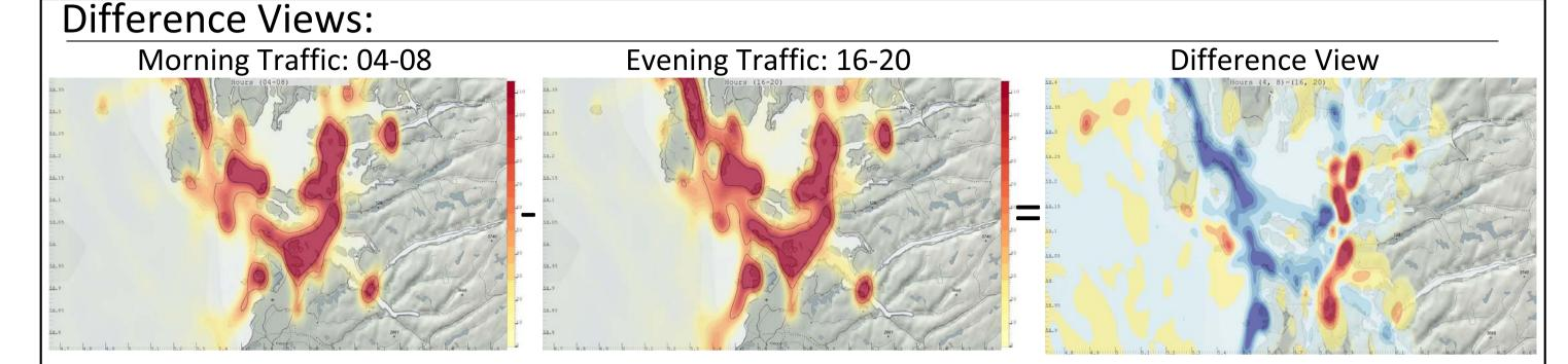
The images show kernel density sum of all ship traffic close to Stavanger in a given time period. These plots gives a good quantitative measurement on the volume of traffic in the different areas. If the user investigates how the traffic volume changes over time, however, a side by side presentation will only provide a qualitative idea on changes.
