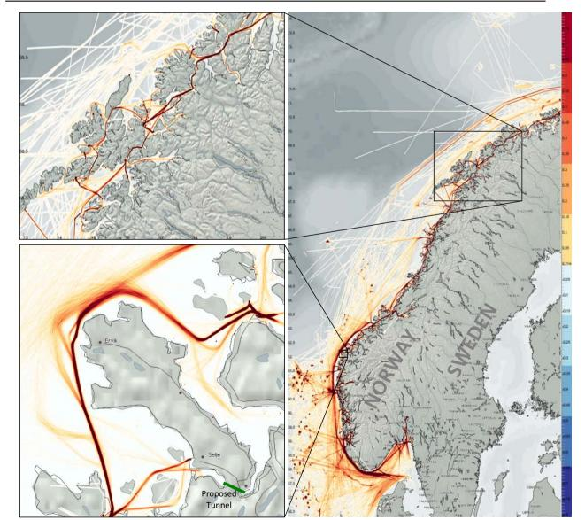
The Automatic Identification System (AIS) collects the position, heading and several other attributes on all vessels close to the coast. The top inset shows how traffic is protected in-shore by a series of islands. The bottom inset shows how the traffic passing Stad is forced to take a route that is exposed to the harsh weather conditions of the North Sea. This inset also shows a proposed tunnel in green, wich would allow traffic to bypass Stad alltogether.
